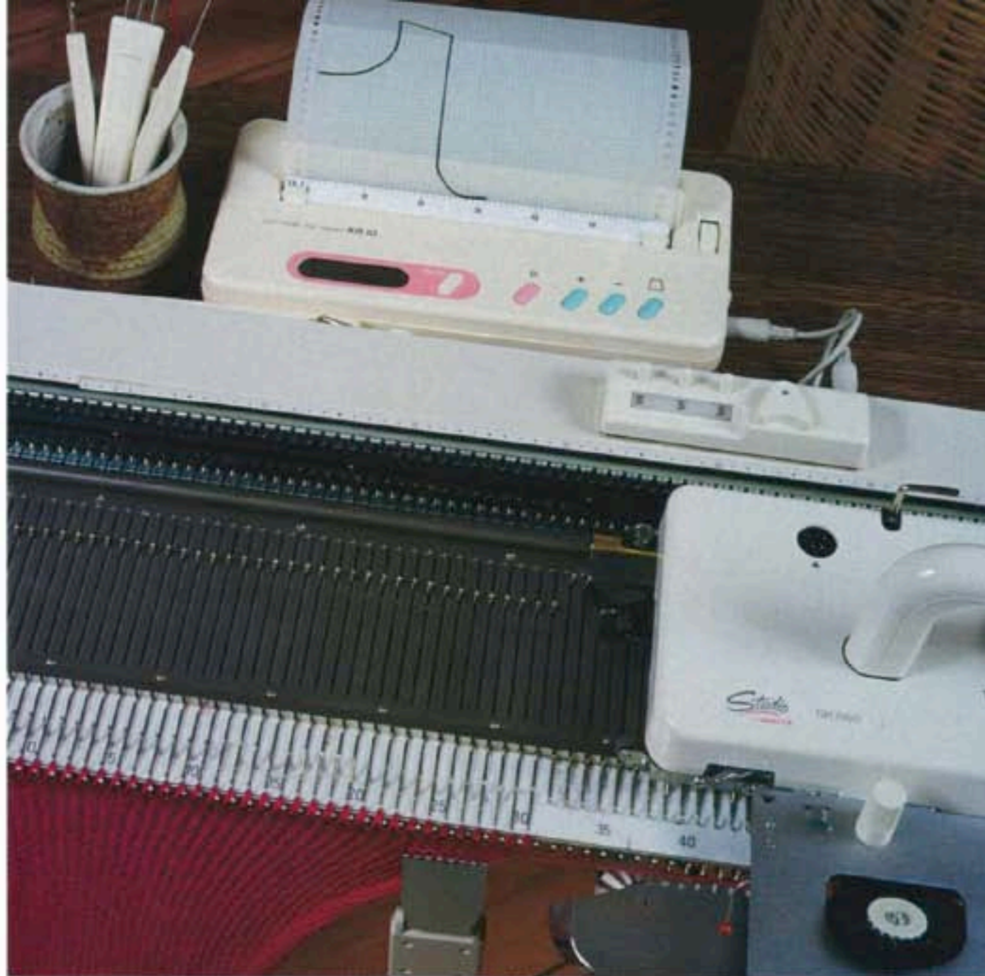
Most knitting machines can be fitted with an ingenious charting attachment that eliminates all the tedium of calculating. All you need is a schematic and a gauge swatch you like. The device shows you when and where to shape or pattern. (Photo by Susan Kahn)
